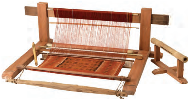
Cagcag (backstrap loom), comprising frame, yoke, shuttle, blade/beater, reed, lease bar, string heddle, and loom cloth Ngurah Hendrawan and Ni Gede Diari, makers. Nusa Penida, Bali, Indonesia. 2017. Wood, bamboo, cotton. Bard Graduate Center Study Collection.
